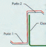
Fixing arrangement of Z-Purlin with Cleat
